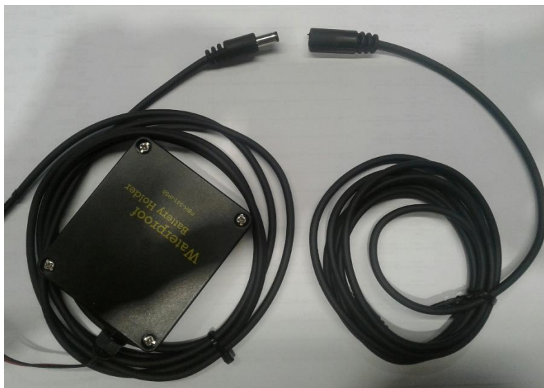
Photo 7 – Battery box connection
