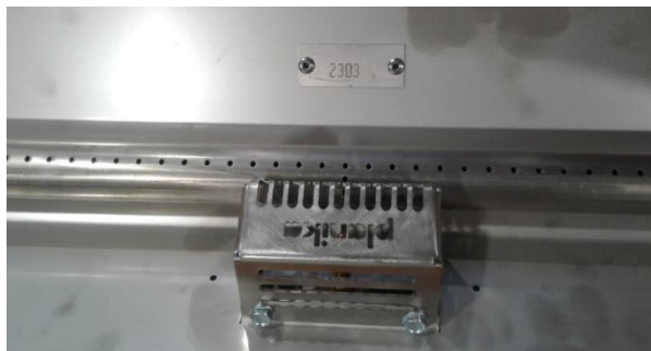
Photo 12 – Wall Switch connection and serial number location
